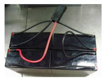
2. As shown left: get 4 batteries in serial connection
