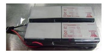
1.As shown left: get the batteries stuck onto the double-side tap on the previous isolation tray
