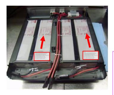
1.As shown both of two: Push the assembled battery bank into the case following the instructed direction (the red arrow)
